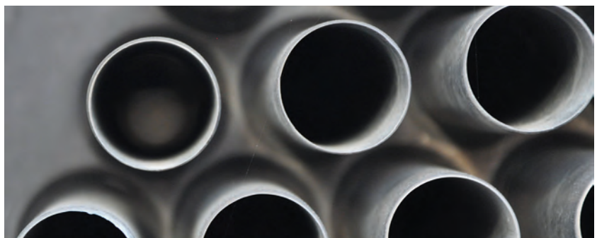
Tubes of a Heating Chamber
